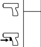
On manual mode, connect the power and trigger command connectors. Automatic mode is disabled, only pressure on the trigger will create the arc. The switch enable to activate or deactivate the trigger gun.
