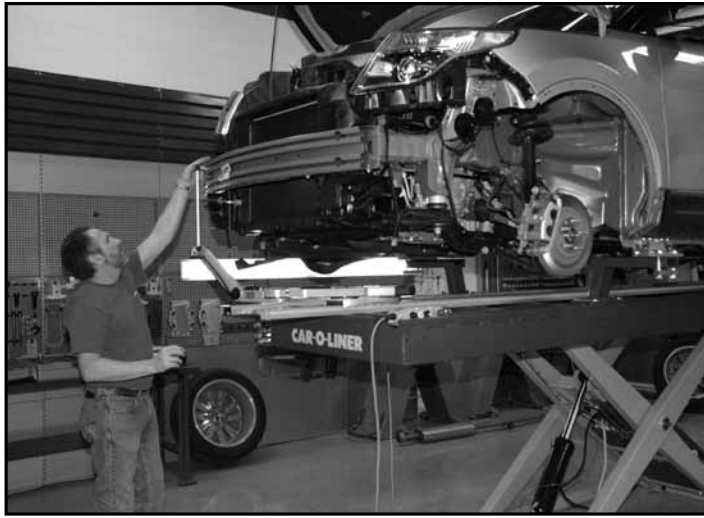
Measure the underbody and upper body with precise measuring and damage analysis.
