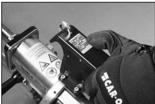
Automatically senses metal type and thickness to set power and tip pressure.
