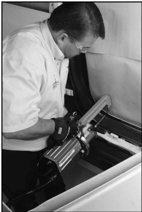
Greater power efficiency via the 10 kHz transformer C-gun.
